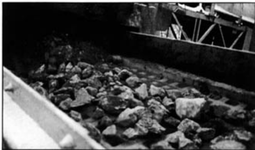
Isenmann urethane scalping screens significantly reduce noise at the primary plant. Wear is comparable to stainless steel.
