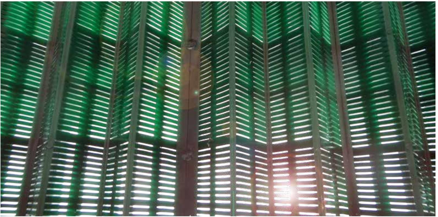
Multotec TeePee™ panels are injection moulded, ensuring repeatable class-leading performance. Computer controlled injection machines maintain optimum conditions throughout the manufacturing process, resulting in consistent aperture sizing in a robust and hard wearing polyurethane.
