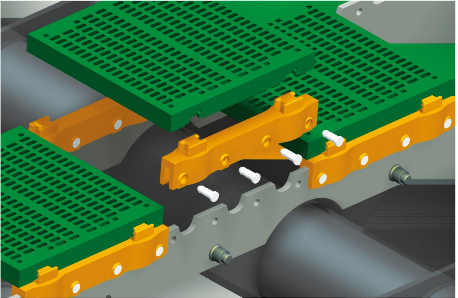
The Multotec P3 Pinless Panel Fastening System simplifies panel maintenance operations. Only the panel and compatible Saddle Top™ are required to fasten the screen panel to the deck. Fewer steps ensure more efficient maintenance and improved operator safety. The P3 system has been designed to have minimal installation and removal forces, yet maximum panel fastening forces to keep the panels in place.
