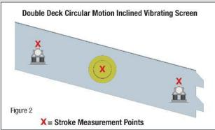
From the information we can determine the gravitational force being generated by the drive of the vibrating screen and whether the screen is structurally sound.
