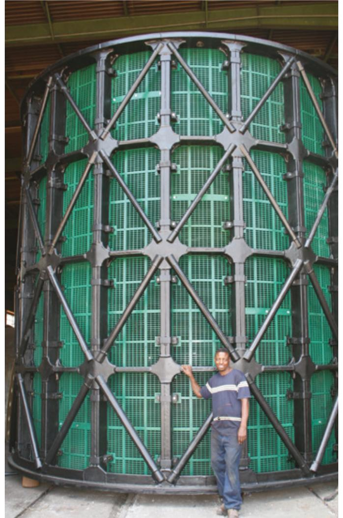
5 000 mm diameter by 5 500 mm long Trommel Screen
