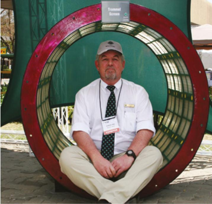
950 mm diameter by 1 220 mm long Trommel Screen
