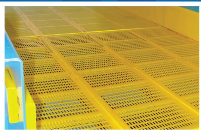
Flex-A-Thon screens are made from a thin, yet highly durable, polyurethane material. The urethane membrane is punched and pretensioned to be lively, flexible and resilient, and provides the highest open area of any synthetic screen.
