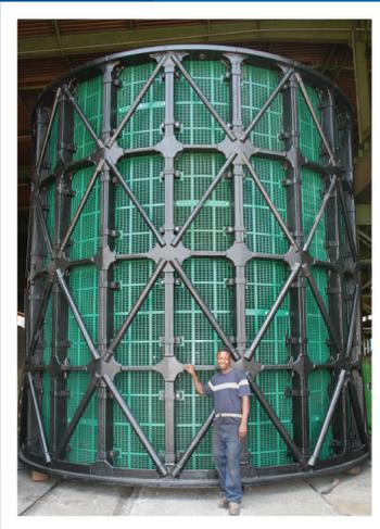
Self-Driven Trommels complete with hydraulic variable speed drive, and range in size from 1000mm to 4500mm in diameter and lengths in excess of 15000mm.
